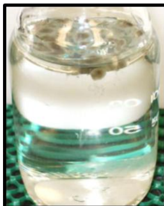
Figure 5: H. resinae growth in Bushnell Haas Medium, augmented with 5% v/v each, Trypticase Soy Broth and Jet A-1 Fuel
