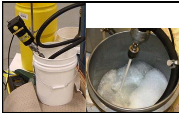
Figure 4: Fuel Reservoir with High-speed Mixer
