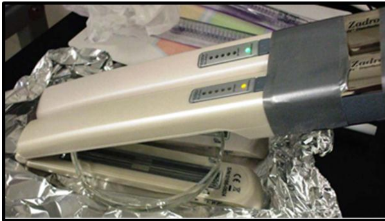
Figure 2: UVm Light Set-up with Jet A-1 in 125 mm dia Quartz Petri Dish
