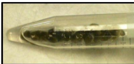
Figure 6: H. resinae Colonies Harvested from Bushnell Haas Broth, Fuel Phase
