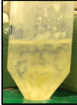
Figure 1: Acinetobacter sp. RAG-1 After Centrifugation for 15 min at 5,000 x g and Attempted Resuspension in Jet A1 Fuel
