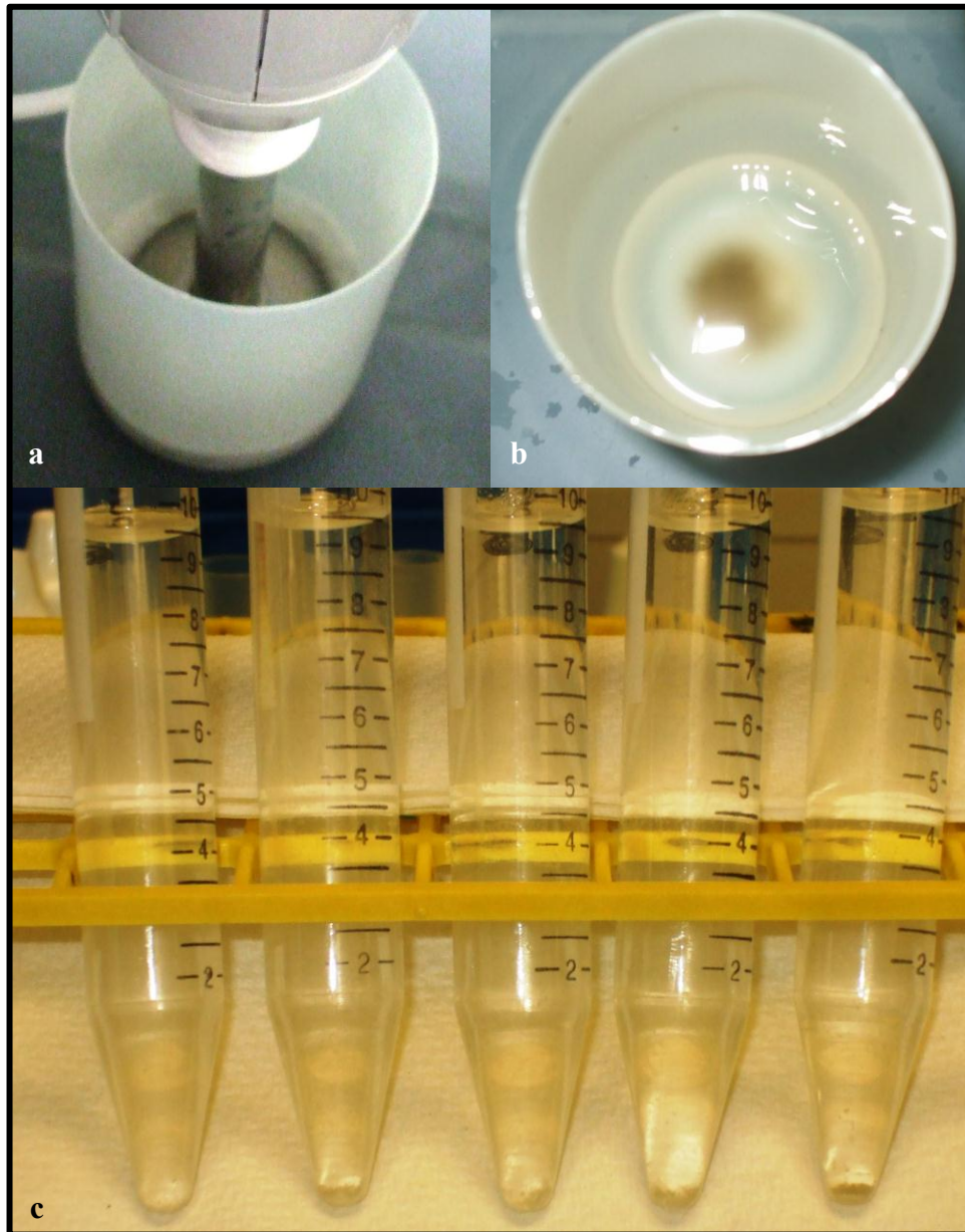
Figure 2: Shearing H. resinae Hyphae with Hand-Held Blender.
